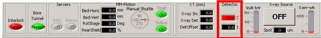
Detector temperature indicator on CT status panel
