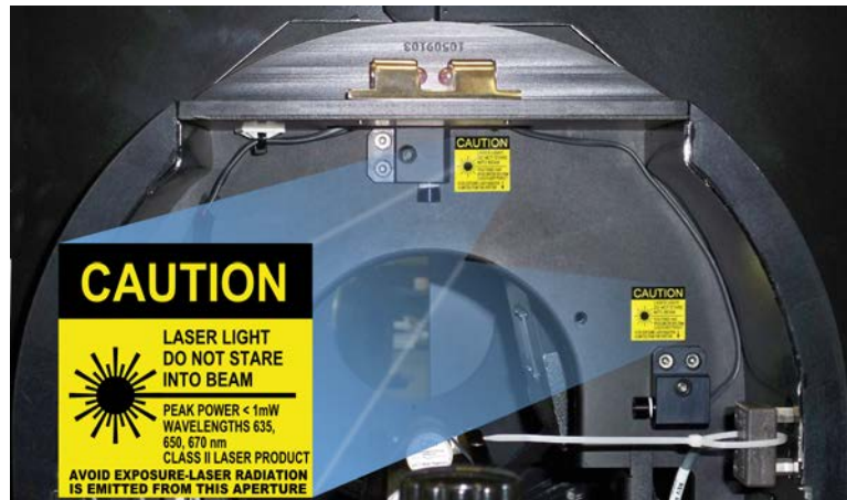
A laser warning label appears by each of the MM's two lasers
