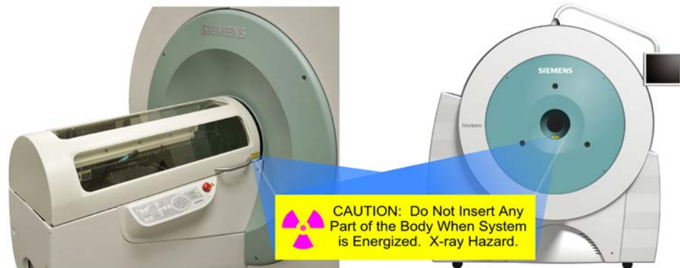
Access port warning labels by each bed cover handle and below the rear shield
