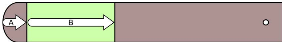
The co-scan length (B) and its distance from the tip of the pallet (A)
