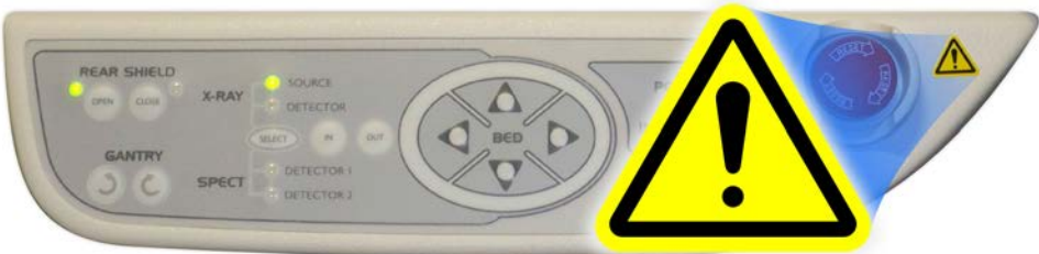
General warning label by the emergency stop button on each control panel
